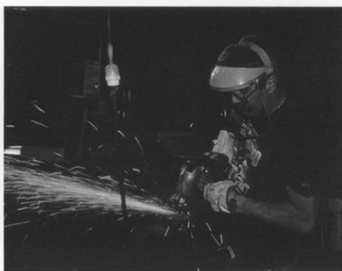
Fig. 8-23. Face shields (secondary protectors) are designed to protect the entire face. They must be worn over industrial safety glasses, as pictured here, or chemical goggles (American National Standards Institute [ANSI] Z87.1-approved primary eye protectors).
